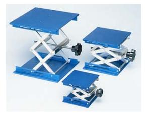
Manufactured to close tolerances from aluminium with stainless steel operating screw. The top and bottom plates are specially designed aluminium extrusion giving exceptional rigid and robust support without excessive weight. The plates are blue anodised finish. The labjacks are designed to be completely stable and free from rocking movements. Labjacks are supplied in blue.
